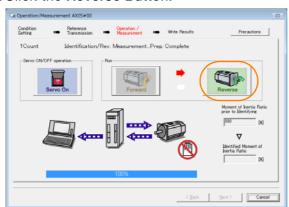
The Servomotor shaft will rotate in the reverse direction and the measurement will start. After the measurement and data transfer have been completed, the **Forward** Button will be displayed in color.
